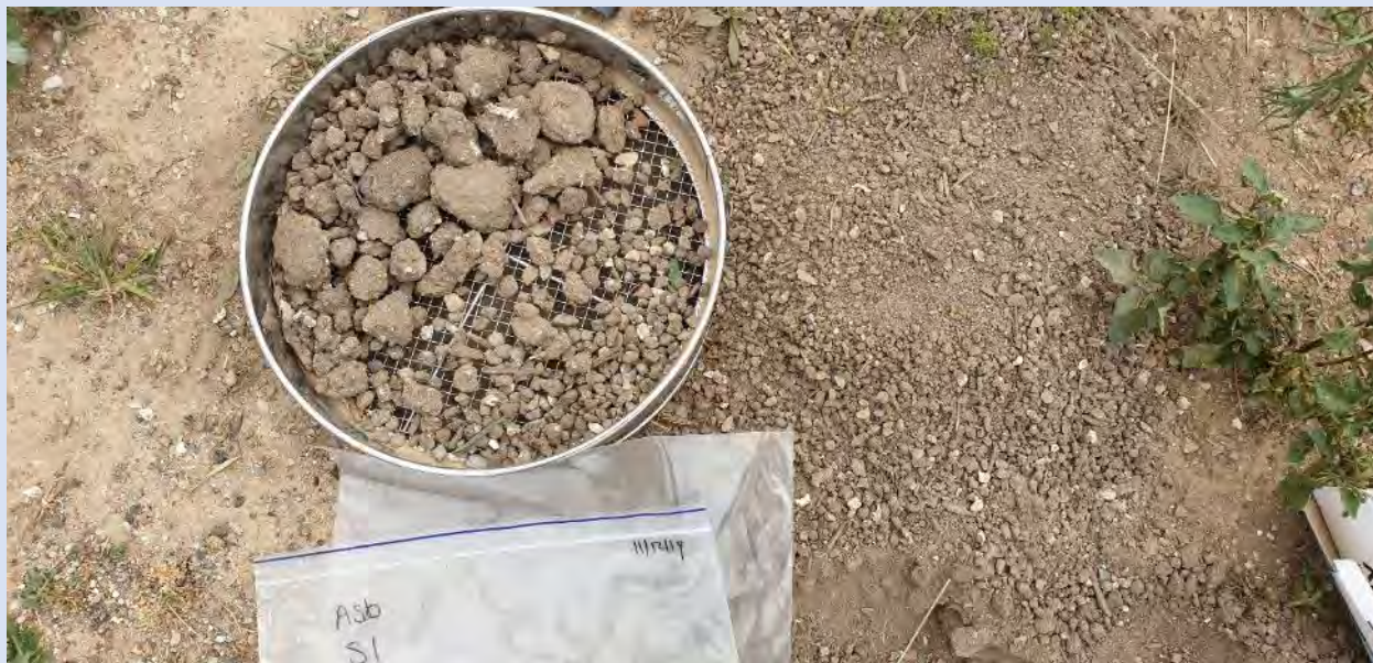
Photograph 15: Asbestos in soil samples sieved to 7 mm
